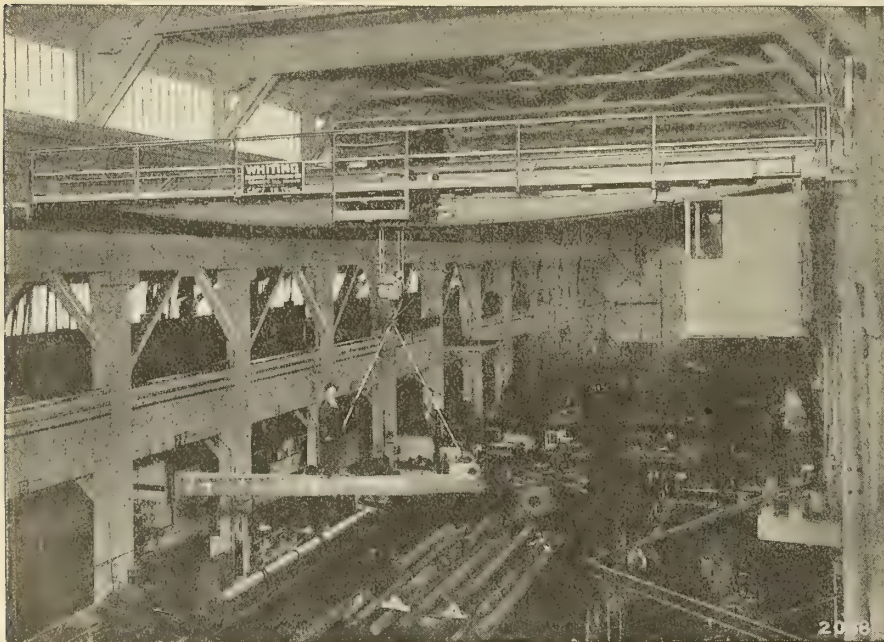
Three-Motor Whiting Electric Traveling Crane Capacity 10 tons, Span 46 ft. Skinner & Eddy Corporation, Seattle, Wash.
